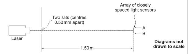
The array of light sensors is connected to circuitry that displays a graph of light intensity along the line AB.
