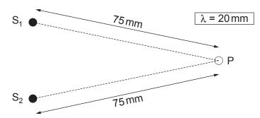
$\rm S_2$  remains stationary while  $\rm S_1$  is made to vibrate up and down, so waves spread outwards from it across the water. The wavelength of the waves is 20 mm. A displacement-time graph is given for point P.
